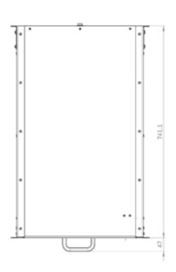
Depth Height Width 306,1 mm + 47 mm Handle 89 mm 483 mm 694,1 mm + 47 mm Handle 89 mm 483 mm
