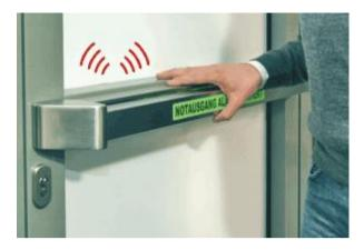
When pushing the e-Bar® completely, the emergency exit door opens and the display emits a flashing green light and a permanent acoustic alarm (95dBA/1 m). Only an authorised person with a key may switch off and reactivate the e-Bar®. An automatic alarm shutdown can be set up.
