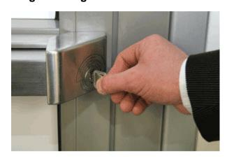
By using the integrated key switch or by employing an external access control system, an authorised person may pass through the emergency exit once. In case the door has been left open for more than 10 seconds a gentle "dooropen too long" alarm is emitted.
